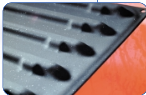
One coat catalytic self clean applied to degreased only steel
